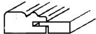
504F - Shown with 115 edge HEIGHTS LESS THAN 5 1/2" WILL HAVE "R" PANEL CUT.
